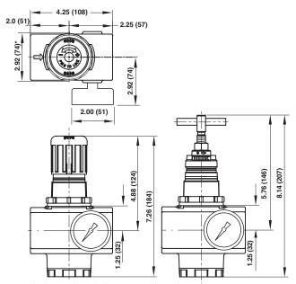
Panel mounting hole diameter: 2.28" (58 mm) Panel thickness: 0.06" to 0.16" (2 to 4 mm) \*OD of panel mount nut. Nut not included
