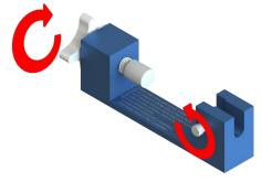
Place the capacitance sensor tip into the go-gauge, then pull the sensor back until the shoulder is captured.
