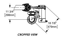
PRODUCT TO BE CONVEYED: ETHANOL SWIVEL SEALS (CONTACTING PRODUCT): FKM GREASE: STANDARD (LITHIUM SEMI-SYNTHETIC)
